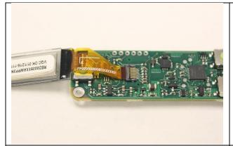
**Step 3:** Fully insert the flexible cable into the front of the socket with the contact side towards the PCB
