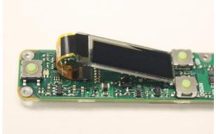
**Step 4:** Close the locking tab and press until the connector gently clicks. Remove the clear screen protector by pulling on the colored tab.
